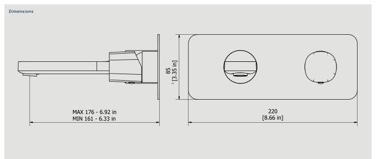
Cartridge Threaded fitting Treaded fitting G1/2" female Ø35 ceramic cartridge Aerator Flow Rate (+/-10%) M24x1 1 BAR 2 BAR 3 BAR 4.5 I\min 5 I\min 5 I\min
