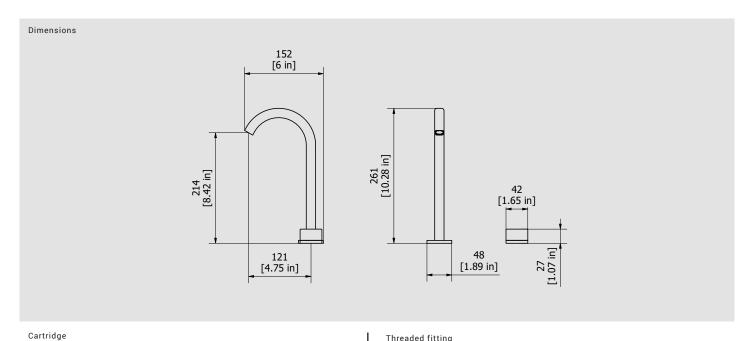
Threaded fitting G1/2" female 400mms Ø25 progressive cartridge Aerator Flow Rate (+/-10%) 1 BAR 2 BAR 3 BAR M16.5x1 3 I\m 3.8 l\m 3.8 I\m
