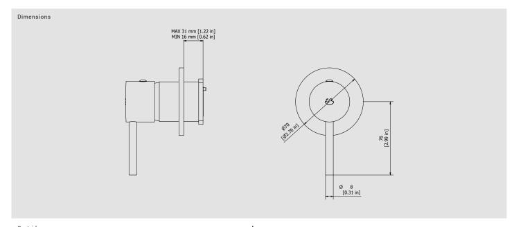
Cartridge Threaded fitting Ø35 ceramic cartridge
