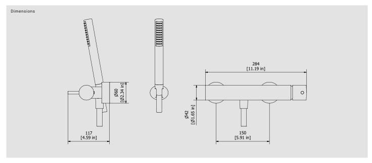
Cartridge Treaded fitting Ø35 ceramic cartridge G1/2" male Aerator Flow Rate (+/-10%) 1 BAR 2 BAR 3 BAR 12.5 l\m 17.4 l\m 21 I\m
