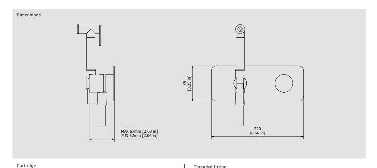
Ø35 Ceramic cartridge Flow Rate (+/-10%) Aerator 1 BAR 2 BAR 3 BAR 2.3 l\m 3.2 l\m 4 I\m
