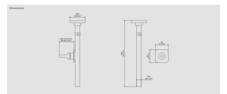
Cartridge Threaded fitting G1/2" male Ceramic cartridge joystick Ø35 Aerator Flow Rate (+/-10%) 1 BAR 2 BAR 3 BAR M16.5x1 4.3 l\m 5.2 I\m 7 I\m
