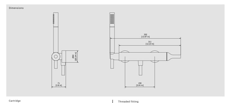
Ceramic cartridge Ø35 G1/2" Aerator Flow Rate (+/-10%)
