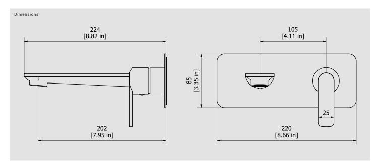
Cartridge Threaded fitting Ø35 ceramic cartridge G1/2" female Aerator Flow Rate (+/-10%) M24x1 1 BAR 2 BAR 3 BAR 3 l\m 3.8 l\m 3.8 l\m
