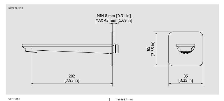
G1/2" male Flow Rate (+/-10%) Aerator 1 BAR 2 BAR 3 BAR M24x1 3 l\m 4 I\m 4 I\m
