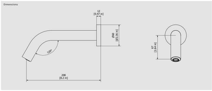
Cartridge Threaded fitting **Tube flex** Aerator Flow Rate (+/-10%) 1 BAR 2 BAR 3 BAR M16.5x1 4.5 l\m 6 I\m 6 l\m
