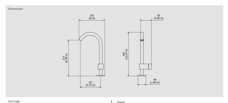
Inox hoses G1/2" female 450mms Ø25 progressive cartridge Aerator Flow Rate (+/-10%) 1 BAR 2 BAR 3 BAR M16.5x1 3 I\m 3.8 I\m 3.8 l\m
