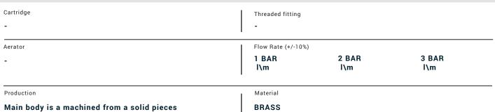
BRASS According to CuZn39Pb3 (CW614N) Max Lead content: 2.5%
