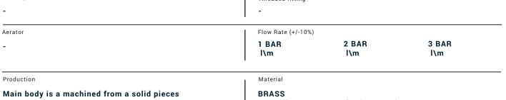
BRASS According to CuZn39Pb3 (CW614N) Max Lead content: 2.5%
