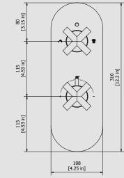
Cartridge Threaded fitting -Flow Rate (+/-10%) Aerator 1 BAR 2 BAR 3 BAR l\m l\m l\m Production Material Main body is a machined from a solid pieces BRASS According to CuZn39Pb3 (CW614N)
