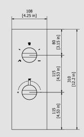
Cartridge Threaded fitting -Flow Rate (+/-10%) Aerator 1 BAR 2 BAR 3 BAR l\m l\m l\m Production Material Main body is a machined from a solid pieces BRASS According to CuZn39Pb3 (CW614N) Max Lead content: 2.5%
