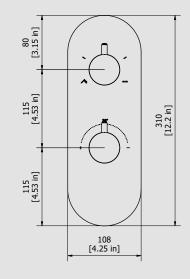
Cartridge Threaded fitting -Flow Rate (+/-10%) Aerator 1 BAR 2 BAR 3 BAR l\m l\m l\m Production Material Main body is a machined from a solid pieces BRASS According to CuZn39Pb3 (CW614N) Max Lead content: 2.5%
