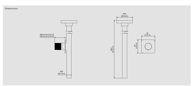
Cartridge Threaded fitting G1/2"M Ø35 ceramic cartridge Aerator Flow Rate (+/-10%) 1 BAR 2 BAR 3 BAR M16.5x1 4.3 l\m 5.2 I\m 6.9 I\m
