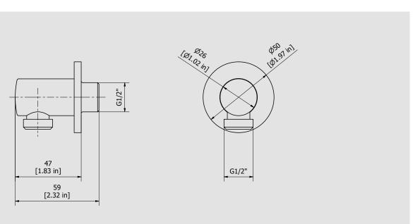
Cartridge Threaded fitting G1/2" male Flow Rate (+/-10%) Aerator 1 BAR 2 BAR 3 BAR - I\m - I\m - I\m
