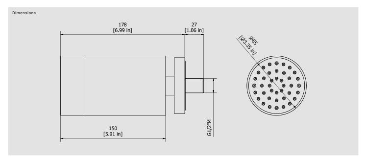
Cartridge Threaded fitting **G1/2**" Male Flow Rate (+/-10%) Aerator 1 BAR 2 BAR 3 BAR 6 I\m 8 I\m 8 I\m
