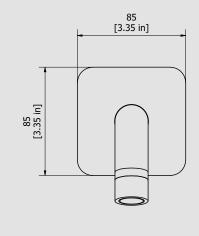
Cartridge Threaded fitting G1/2" male Aerator Flow Rate (+/-10%) 1 BAR 2 BAR 3 BAR M24x1 6.5 l\m 8 I\m 8 l\m Production Material Main body is a single hot stamped pieces BRASS According to CuZn42 (CW510L) Max Lead content: 0.2%
