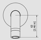
Cartridge Threaded fitting G1/2" male Aerator Flow Rate (+/-10%) 1 BAR 2 BAR 3 BAR M24x1 17.5 l\m 23 I\m 29 I\m Production Material Main body is a single hot stamped pieces BRASS According to CuZn42 (CW510L) Max Lead content: 0.2%
