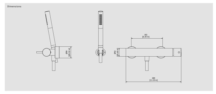
Cartridge Threaded fitting Ø35 ceramic cartridge G1/2" male Flow Rate (+/-10%) Aerator 3 BAR 1 BAR 2 BAR 12.5 l\m 17.5 l\m 21 I\m
