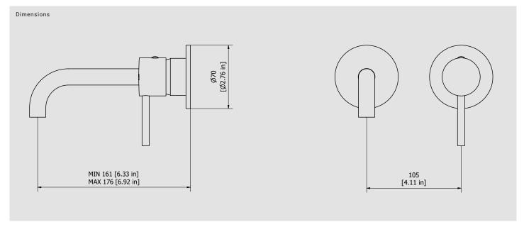
Cartridge Threaded fitting G1/2" female Ø35 ceramic cartridge Aerator Flow Rate (+/-10%) 1 BAR 2 BAR 3 BAR M16.5x1 3 I\m 3.8 I\m 3.8 I\m
