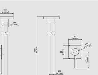
Cartridge Threaded fitting G1/2" male Ø35 ceramic cartridge Aerator Flow Rate (+/-10%) 1 BAR 2 BAR 3 BAR M18.5x1 4.3 l\m 5.2 I\m 7 I\m
