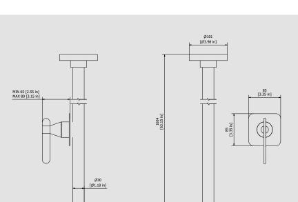
G1/2" male Ø35 ceramic cartridge Aerator Flow Rate (+/-10%) 1 BAR 2 BAR M24x1
