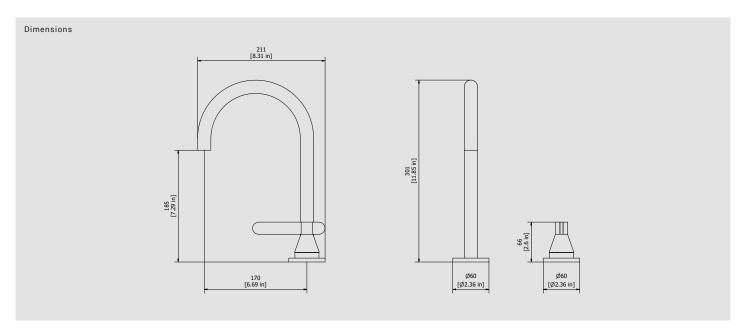
Cartridge Treaded fitting G3/4" female Ø35 ceramic cartridge Aerator Flow Rate (+/-10%) 1 BAR 2 BAR 3 BAR M16.5x1 3 I\m 3.8 l\m 3.8 I\m
