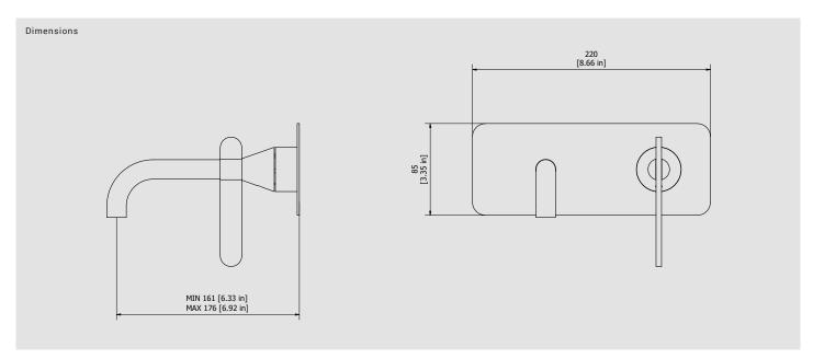
Cartridge Threaded fitting G1/2" male Ø35 ceramic cartridge Aerator Flow Rate (+/-10%) 1 BAR 2 BAR 3 BAR M16.5x1 3 I\m 3.8 l\m 3.8 I\m
