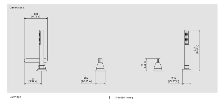
Inox hoses G1/2" F L300 Ø35 ceramic cartridge Aerator Flow Rate (+/-10%) 1 BAR 2 BAR M24x1
