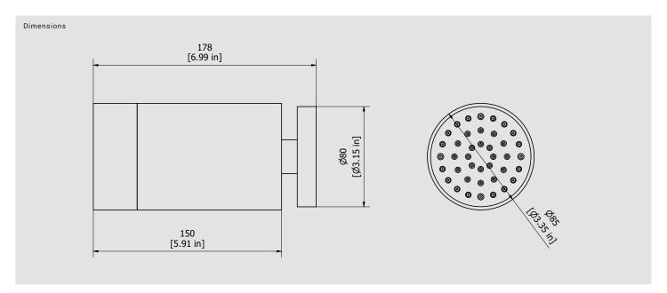
Cartridge Threaded fitting **G1/2**" Male Flow Rate (+/-10%) Aerator 1 BAR 2 BAR 3 BAR 6 I\m 8 I\m 8 I\m
