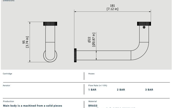
According to CuZn39Pb3 (CW614N) Max Lead content: 2.5%
