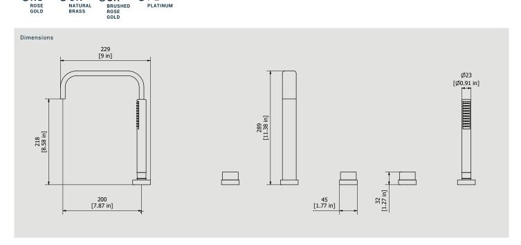
Cartridge Threaded fitting G1/2" male G1/2" ceramic cartridge Aerator Flow Rate (+/-10%) 1 BAR 2 BAR 3 BAR 21 I\min 29 I\min 36 I\min
