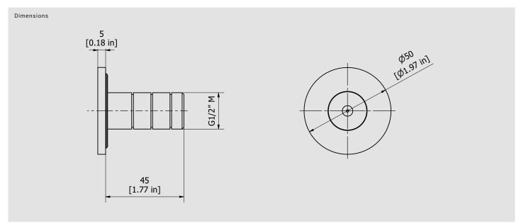
Cartridge Threaded fitting G1/2" M Flow Rate (+/-10%) Aerator 1 BAR 2 BAR 3 BAR 1 I\m 2 I\m 2 I\m
