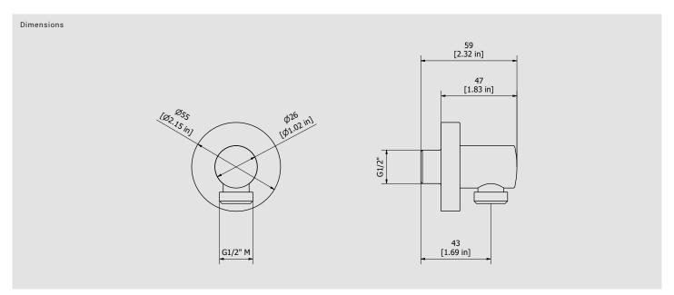
Cartridge Threaded fitting G1/2" male Flow Rate (+/-10%) Aerator 1 BAR 2 BAR 3 BAR - I\m - I\m - I\m
