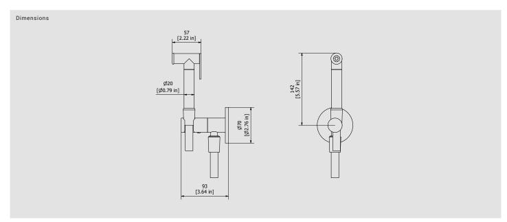
Cartridge Threaded fitting G3/4" ceramic headwork G1/2" male Flow Rate (+/-10%) Aerator 1 BAR 2 BAR 3 BAR 2.3 l\m 3.2 l\m 4 I\m
