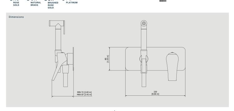
Cartridge Hose G1/2" female Ø35 ceramic cartridge Aerator Flow Rate (+/-10%) 1 BAR 2 BAR 3 BAR 2.3 I\min 3.2 I\min 4 I\min
