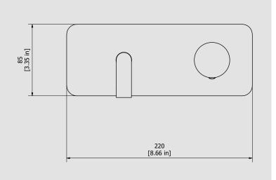
Cartridge Threaded fitting G1/2" female Ø35 ceramic cartridge Aerator Flow Rate (+/-10%) 1 BAR 2 BAR 3 BAR M16.5x1 3 I\m 3.8 I\m 3.8 I\m
