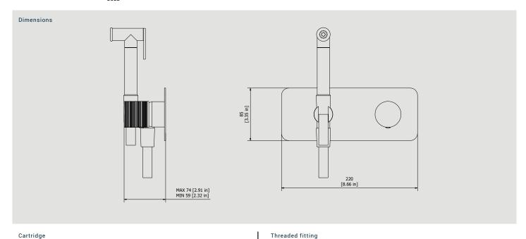
G1/2" female Ø35 ceramic cartridge Aerator Flow Rate (+/-10%) 3 BAR 1 BAR 2 BAR 2.3 I\min 3.2 I\min 4 I\min
