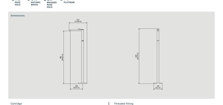
G1/2" female Ø25 ceramic cartridge Aerator Flow Rate (+/-10%) M24x1 1 BAR 2 BAR 3 BAR 3.6 I\min 5.1 I\min 5.5 I\min
