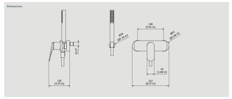
Cartridge Hoses G1/2" male Ceramic cartridge Ø25 Aerator Flow Rate (+/-10%) 1 BAR 2 BAR 3 BAR 5.1 I\min 7.4 I\min 9.1 I\min
