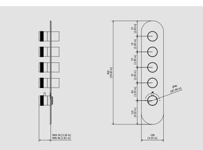
Cartridge Threaded fitting \_ \_ Flow Rate (+/-10%) Aerator 1 BAR 2 BAR 3 BAR l\m l\m l\m Production Material Main body is a machined from a solid pieces
