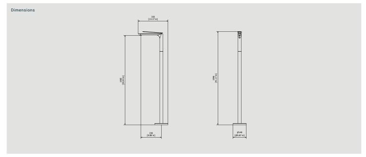
Threaded fitting Cartridge G1/2" male Ø25 ceramic cartridge Aerator Flow Rate (+/-10%) M24x1 1 BAR 2 BAR 3 BAR 3.9 I\min 5 I\min 5 I\min
