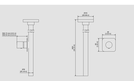
Cartridge Threaded fitting G1/2"M Ø35 ceramic cartridge Aerator Flow Rate (+/-10%) 1 BAR 2 BAR 3 BAR M16.5x1 4.3 l\m 5.2 I\m 6.9 I\m
