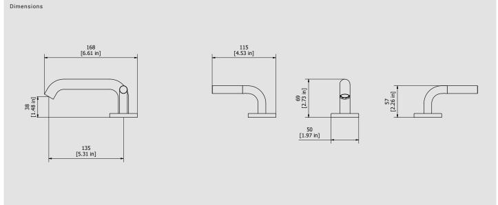
Cartridge Threaded fitting G1/2" ceramic headwork G1/2" male Aerator Flow Rate (+/-10%) 1 BAR 2 BAR 3 BAR M16.5x1 5.5 l\m 6 I\m 6 l\m
