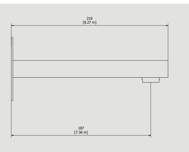
Threaded fitting Cartridge G1/2" male Flow Rate (+/-10%) 2 BAR 3 BAR M24x1 1 BAR 10 I\min 14 I\min 17 I\min
