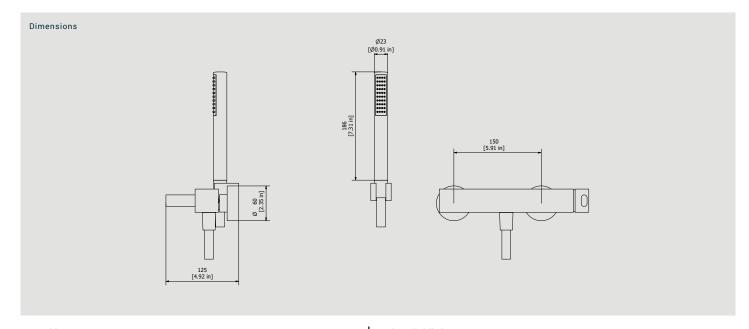
Threaded fitting Cartridge G1/2" male Ø35 ceramic cartridge Aerator Flow Rate (+/-10%) 1 BAR 2 BAR 3 BAR 12.5 I\min 18 I\min 21 I\min
