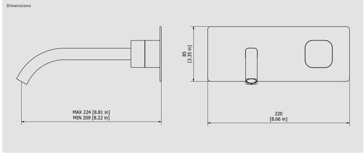
Cartridge Threaded fitting G1/2" male Ø35 ceramic cartridge Aerator Flow Rate (+/-10%) 1 BAR 2 BAR 3 BAR M16.5x1 3 I\m 3.8 l\m 3.8 I\m
