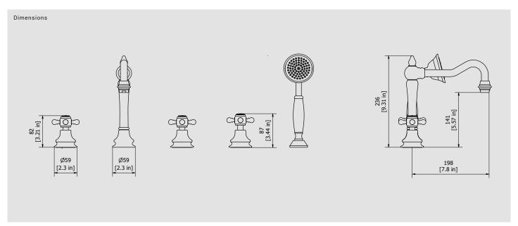
IB G1/2" ceramics headworks Treaded fitting G1/2" male Aerator Flow Rate (+/-10%)
