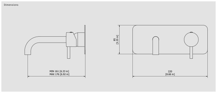
Cartridge Threaded fitting G1/2" female Ø35 ceramic cartridge Aerator Flow Rate (+/-10%) 1 BAR 2 BAR 3 BAR M16.5x1 3 I\m 3.8 l\m 3.8 l\m
