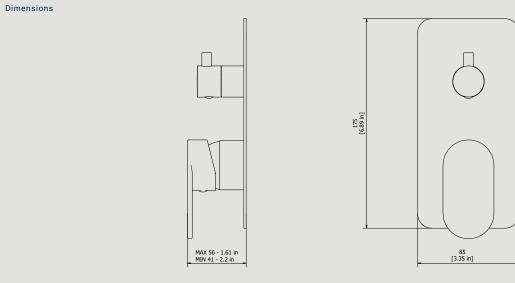
Cartridge Threaded fitting Ø35 ceramic cartridge
