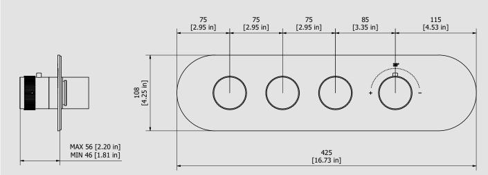
Cartridge Threaded fitting -Flow Rate (+/-10%) Aerator 1 BAR 2 BAR 3 BAR l\m l\m l\m Production Material Main body is a machined from a solid pieces BRASS According to CuZn39Pb3 (CW614N) Max Lead content: 2.5%
